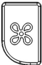
If you press the button with the fan icon, if heating is active, the heater will change the heating level. You can set the maximum, medium and economic heating.
