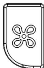
If you press the button with the fan icon, if the fan is active, the heater will change the fan level. You can set the maximum, medium, and minimum speed.
